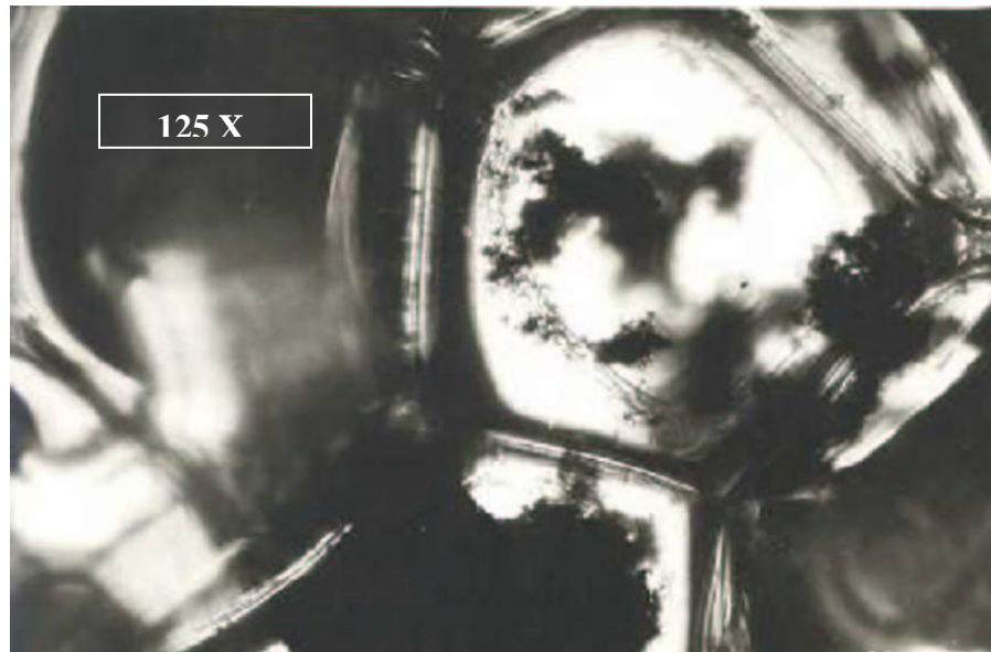
Figure 11 Media @ 125X showing loose flocs in the interstitial volume
